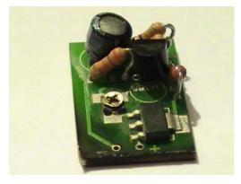
current in milivolts. If you are reading 300mv across R1, your output current is 300ma. You can then adjust the potentiometer to adjust current to the desired level. Once you have reached your desired current, you can remove your load and swap out for your laser diode.
